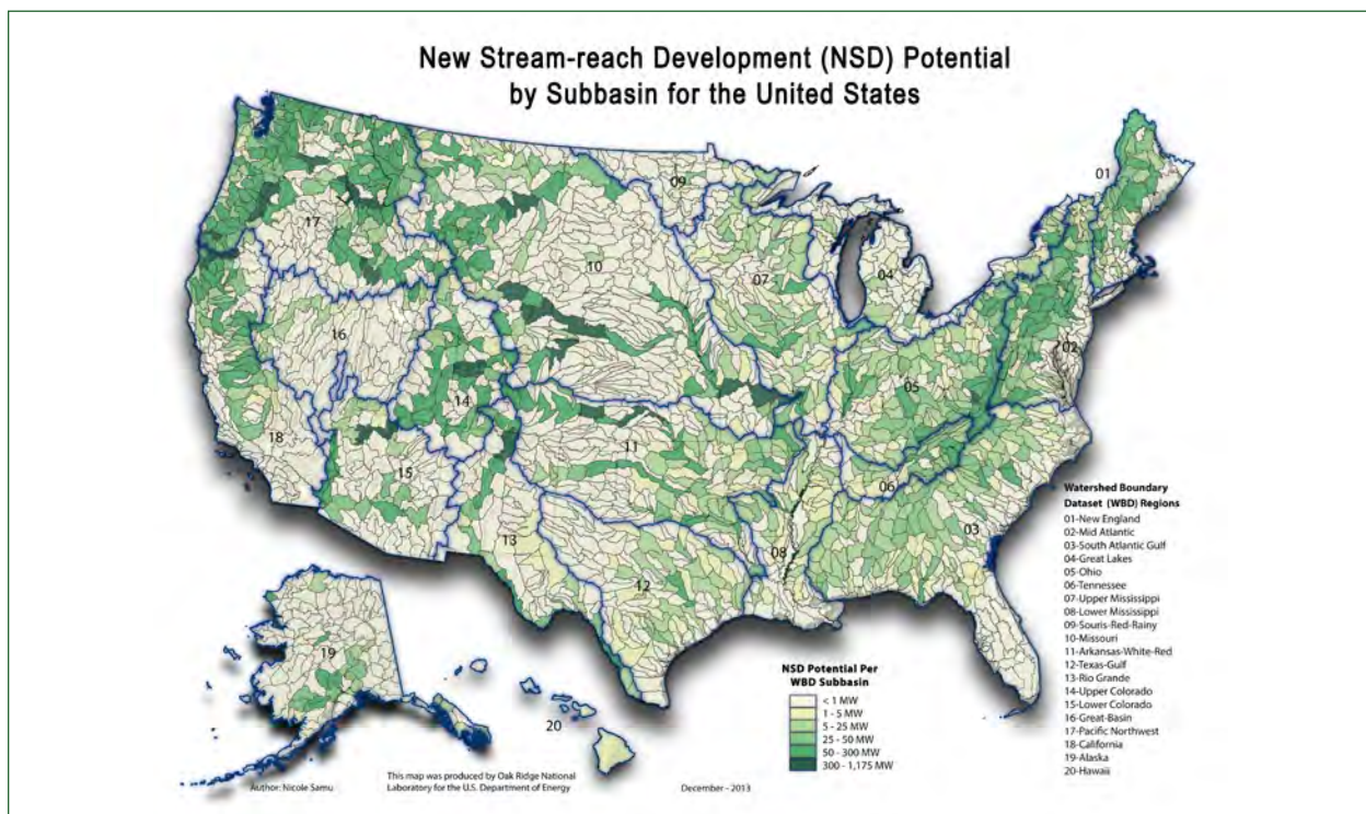
Figure 15: New Stream-reach Development (NSD) potential by U.S. sub-basin. The NSD assessment identifies high-energy intensity stream-reaches and classifies new potential areas for hydropower development using a range of technical, socio-economic, and environmental characteristics.
