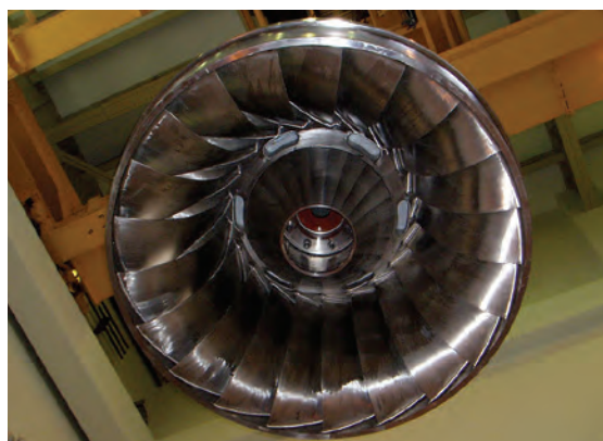
Figure 4: Reassembly of Kortes unit 3 after turbine runner replacement.
